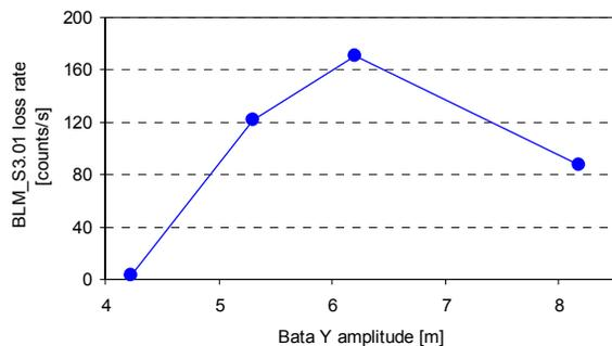
Figure 6: Losses at the wiggler vacuum chamber as a function of the vertical beta function.
