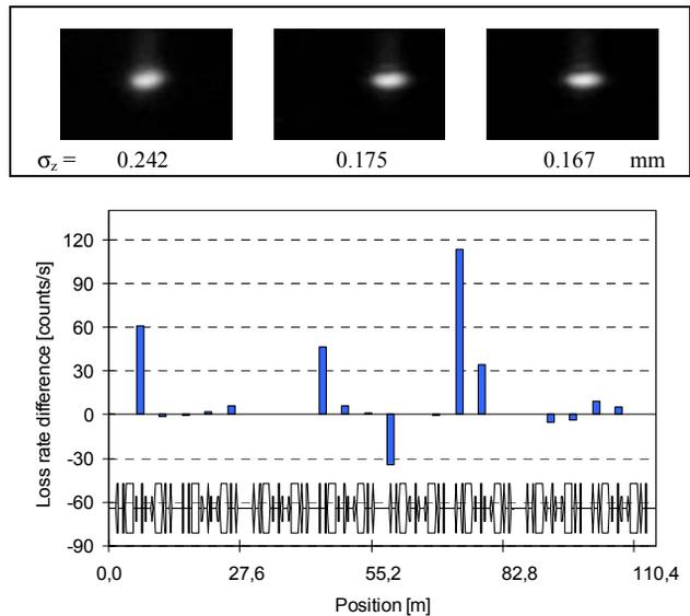
Figure 5: Touschek dominated points, by measuring the difference in loss rate for different vertical beam sizes (top).
