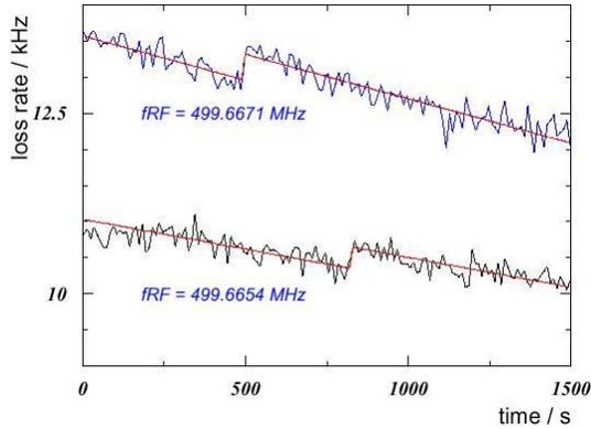
Figure 3: Energy determination by measuring the electron spin precession frequency with the help of the Pb-glass detector.
