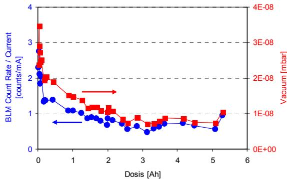
Figure 4: Average vacuum and electron losses as a function of the accumulated Ah dose.
