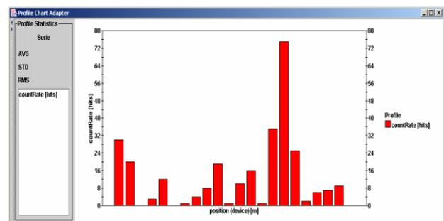
Figure 2: Loss rate at each PIN Diode Detector as seen in the control room.
