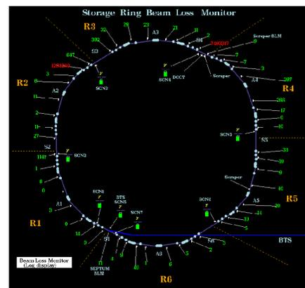
Figure 2. Loss counts display with the storage ring layout.
