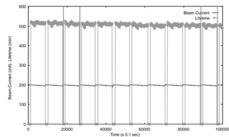
(a) Beam current and lifetime for top-off mode test at 1.3 GeV
