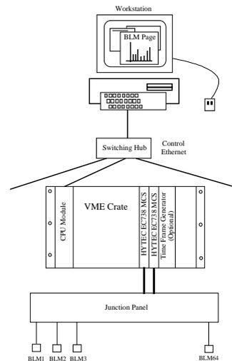
Figure 1. Functional block diagram of beam loss monitoring system
