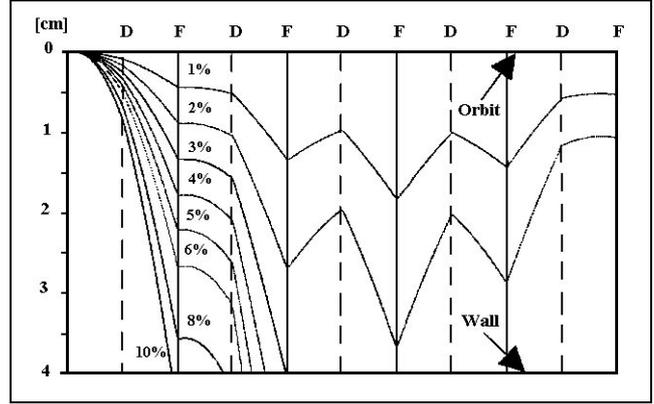
Figure 2: Path of electrons after energy losses. The deviation from the nominal energy is given in %. The vacuum wall starts at 4 cm in HERAe.
