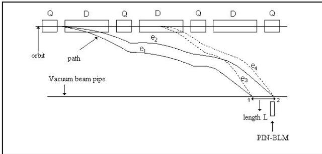
Figure 3: Path of electrons with by  $L$  defined energy losses after Bremsstrahlung at different locations (not in scale).  $e_{1,3}$  and  $e_{2,4}$  represents  $e_{\min}$  and  $e_{\max}$ .
