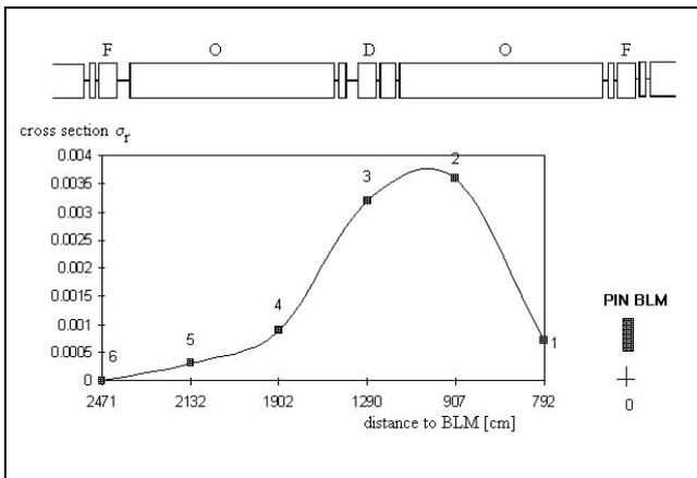
Figure 4: Cross section  $\sigma_r$  along a FODO cell in the arc.
