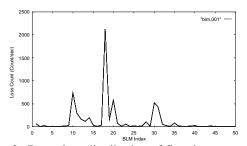
Figure 3. Beam loss distribution of first beam store on April 10, 1997 (beam current 16 mA). The ordinate shows the location of the monitor, and the abscissa shows the count rate.
