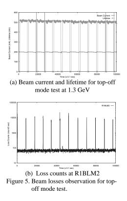
Top-off mode injection has been test in early 1996. Figure 5(a) shows beam current and lifetime during the test. Figure 5(b) shows the loss counts observed by R1BLM2. Loss peaks occur at the instant of injection. Discontinuity on lifetime display is due to the reasons that lifetime calculation is stop during injection and the data length for lifetime estimation needs aabout 3 minute to produce the fist lifetime data.
