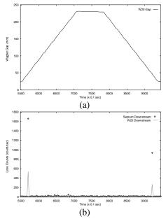
Figure 6. Resonance line crossing during W20 change gap. (a) Wiggler gap; (b) Loss count of BLM at downstream of septum and wiggler.
