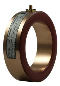
In-air FCTs are typically installed over a vacuum chamber whose wall current flow is interrupted by a user-installed break ("gap") protected from stress by bellows. The wall current is diverted by a user-installed wall current bypass. A user-installed shield prevents RF fields radiating out of the gap.
