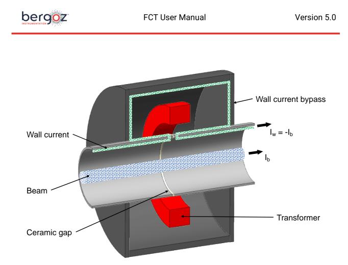
The transformer "sees" all currents passing through its aperture, i.e. beam current  $I_b$  and high frequency components of wall current  $I_w$ . Since these two currents cancel each other, only the beam current components whose corresponding wall current is diverted over the wall current bypass and the high frequency resonances are visible to the transformer. Only these currents induce a magnetic flux in its core.
