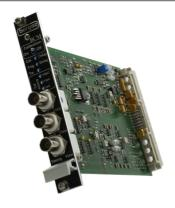
**BCM-IHR-E** inserts into a wired station of BCM-RFC, the 19" 3U RF-shielded chassis including power supplies.
