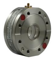
In-flange ICT are mounted directly in the beam line. UHV compatible. Available for many pipe diameters from 1" to 250mm. Also with elliptical aperture or other arbitrary shape aperture. Ceramic gap, shields and wall current bypass are included. Bellows are not required.
