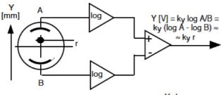
The position of the beam from rotated pickups is obtained by axes translation to the vertical resp. horizontal plane by wideband analog circuits.
