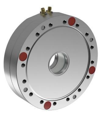
These current transformers are UHV compatible at least to 1e-9 mbar. Soap or alcohol cleaning before installation is however recommended. To reach pressure down to 1e-11 mbar, adequate pumping and prior cleaning, e.g. plasma, are required.
