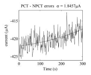
Figure 2: Difference between PCT and NPCT with 500 mA stored. The 420  $\mu$ A offset can be zeroed out.
