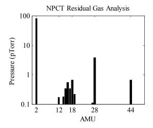
Figure 1: RGA after completion of all vacuum processing.
