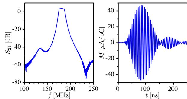
Figure 1: Typical Turbo-ICT response in frequency-domain (left) and in time-domain (right).
