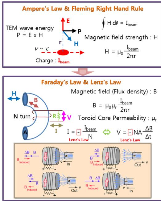
Figure 7: Physical principle of ICT.
