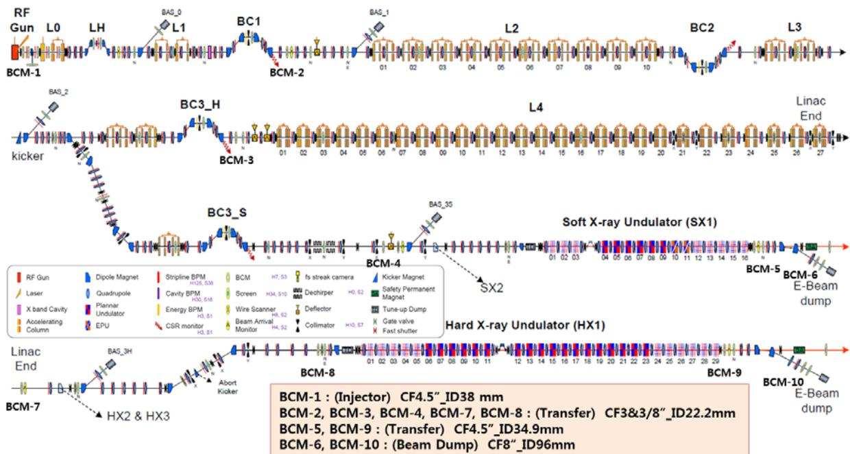
Figure 2: Locations of BCM installed on PAL-XFEL.
