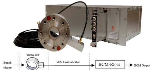
Figure 9: Simplified diagram of a Turbo-ICT.
