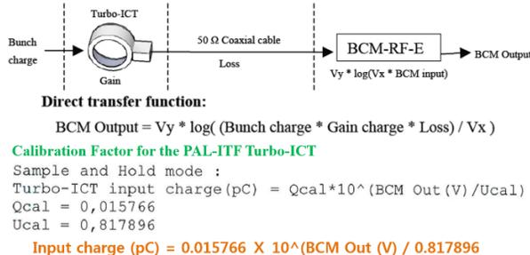
Figure 13: Calculation formula of Turbo-ICT charge amount.
