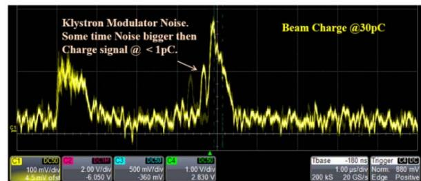
Figure 16: Influence of Klystron modulator Noise.
