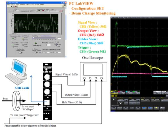
Figure 12: Configuration set and charge monitoring.
