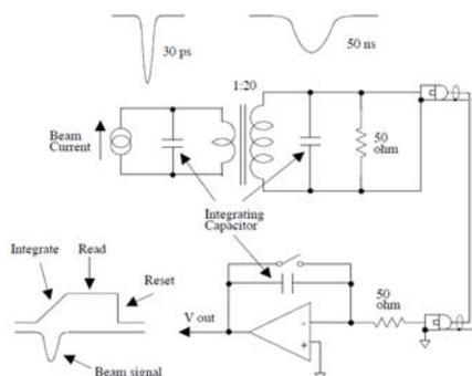
Figure 5: Simplified diagram of a BCM.
