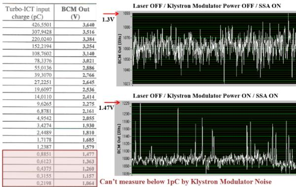
Figure 17: Problems of Klystron modulator noise and measured value of Turbo-ICT on PAL-ITF.
