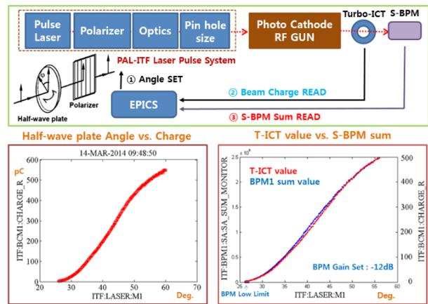
Figure 15: Turbo-ICT following charge control by laser system and BPM Sum value measurement results.
