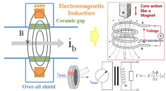
Figure 6: Concept of core induction in the magnetic field generated in an electron beam.
